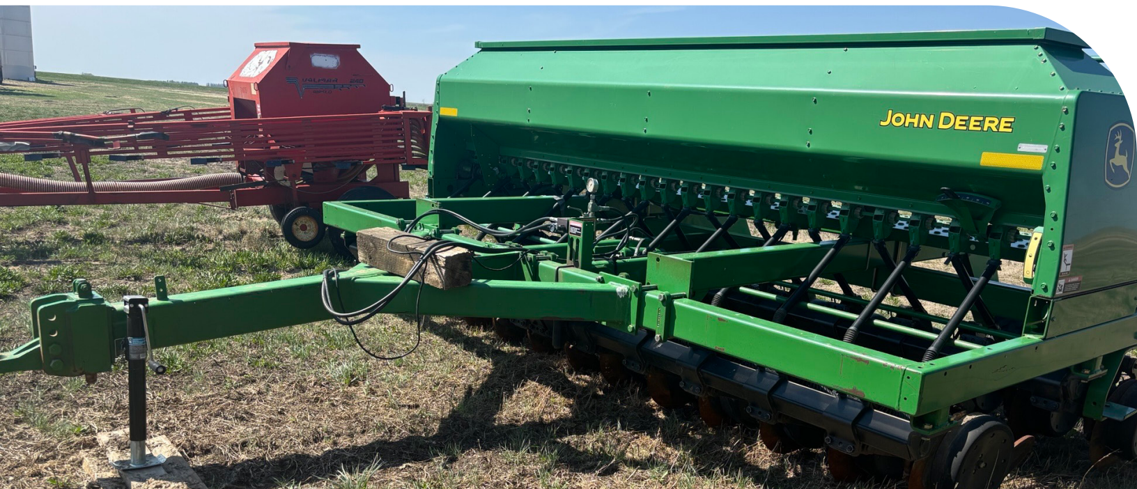
Figure 7: Valmar applicators (red, rear) are used for overseeding by broadcasting seed onto the soil surface. No-till drills, such as the John Deere in the foreground, place the seed directly in the soil. Photo credit: Regan Ferguson
