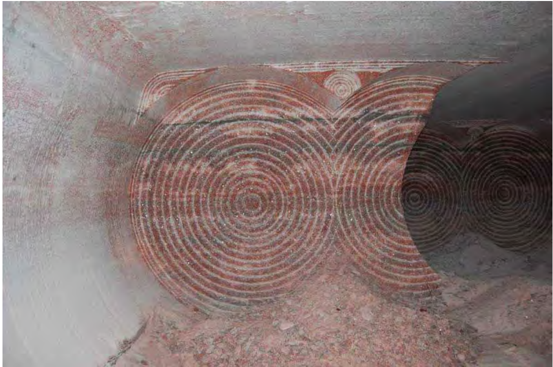
Figure 14: Continuous Mining Operation Face 25
