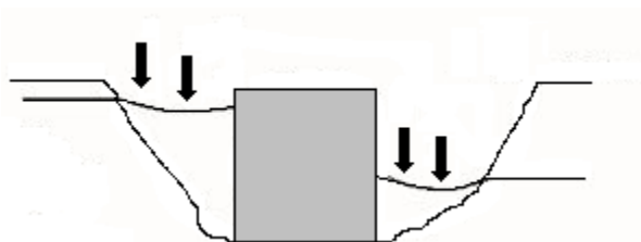
Figure 12-4 - Excessive Tank Excavation
